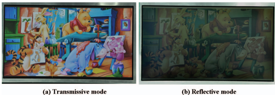
Figure 5. Real Image of Switchable Transmissive and Reflective LCD at (a) transmissive mode and (b) reflective mode.
